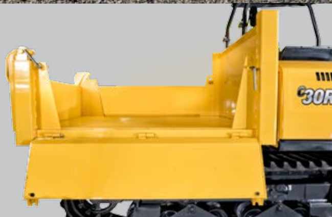
Three-side flaps wagon with rear dumping
