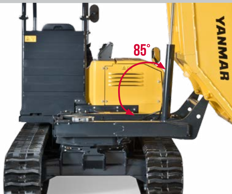
Turning wagon with 180° rotation
