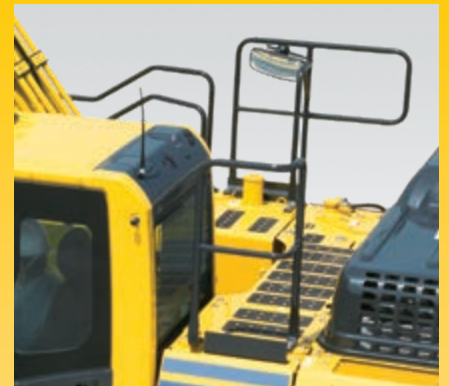
Hand rails and anti-slip plates
